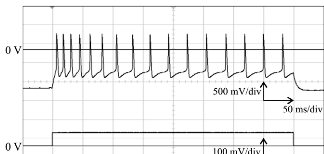
Fig. 8. Excitatory (RS) neuron activity computed and measured on the analog hardware (“Trieste” ASIC). The lower trace is the input voltage, controlling I_{STIM} , applied to the ASIC. The upper trace shows variations of the neuron membrane voltage in response to the stimulation current I_{STIM} .
