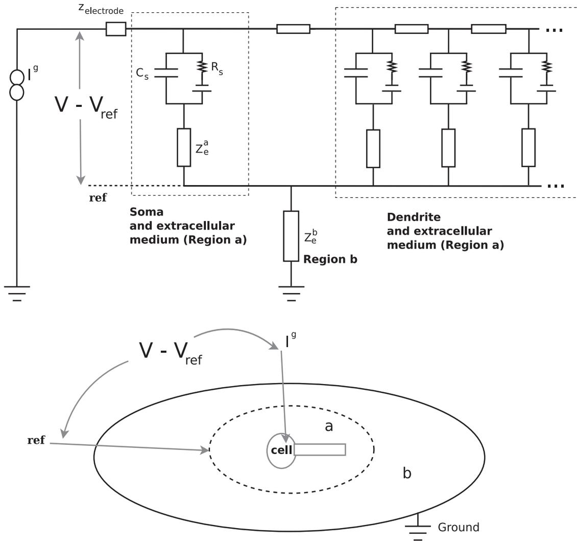
FIGURE 1 Equivalent circuit for the impedance measurements of Gomes et al. (1). A first electrode injects current intracellularly, and the current flows to an electrode in the bath. Another electrode (micropipette) measures the extracellular potential passively and was used as a reference to calculate the impedance. The current flows through the soma membrane as well as the dendritic membrane, as indicated (see (17)).
